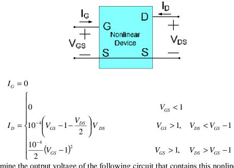
Determine the output voltage of the following circuit that contains this nonlinear device.
